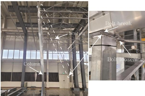
Fig. 5. The failure mode of specimens with bracing members installed in the column top.
