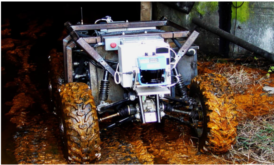
Fig. 3. View of autonomous driving vehicle platform ‘Ground hog’ designed for surveying and mapping in underground mines (Baker et al. , 2004).
