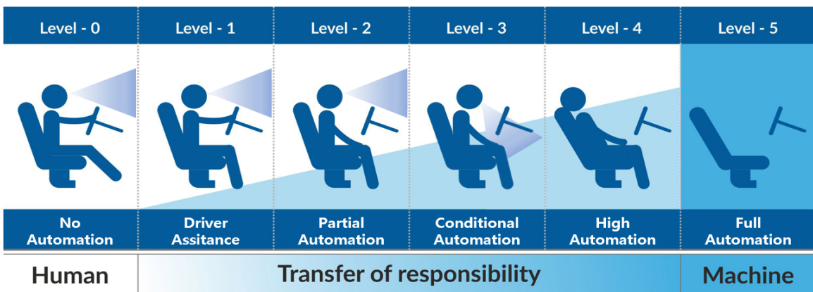
Fig. 1. Levels of autonomous driving technology determined by The Society of Automotive Engineers (modified from NetApp, 2019).
