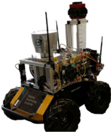
Fig. 4. View of autonomous driving vehicle ‘Barney’ designed for underground mine mapping (Neumann et al. , 2014).
