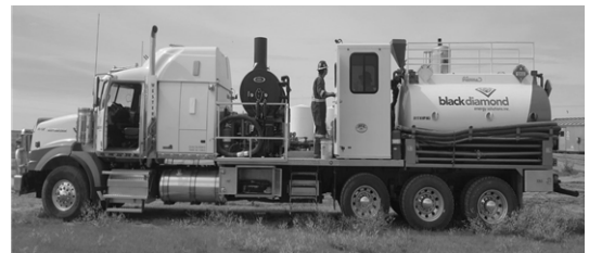
Fig. 6. Water hit & pump operation vehicle for pre-flush.
