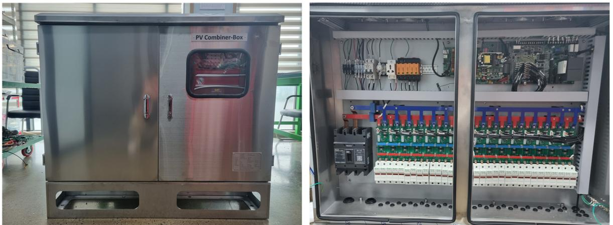
Fig. 2 Internal and external figure of the PV combiner box (left: external, right: internal)
