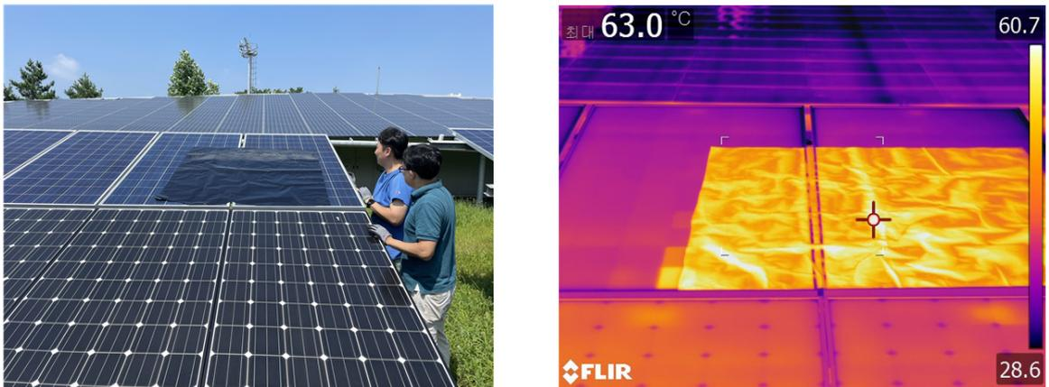
Fig. 6 Induce the Partial shading condition
