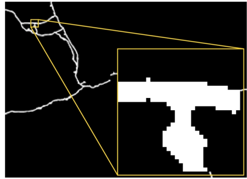
(b) Crack detection image with denoising
