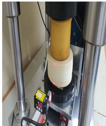
(e) Shear box installation
