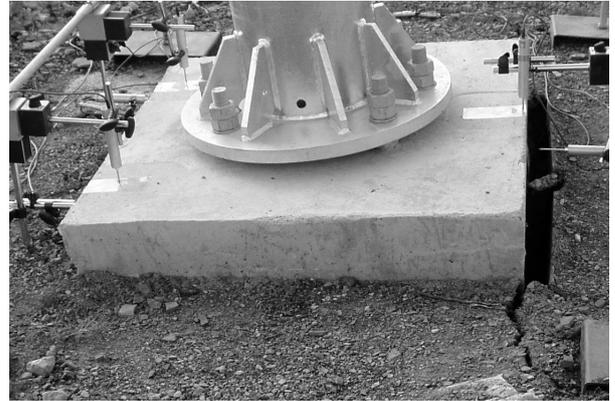
Fig. 12. Horizontal displacement after the foundation failure
