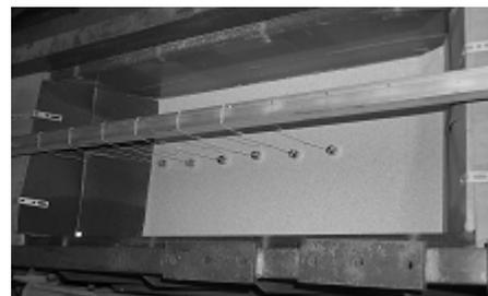
Photo 4. Settlement monitoring apparatus
