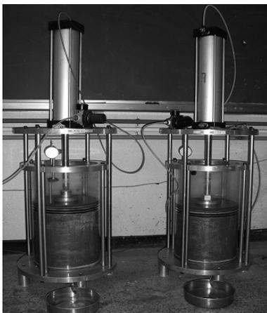
Fig. 2. Preconsolidation test
